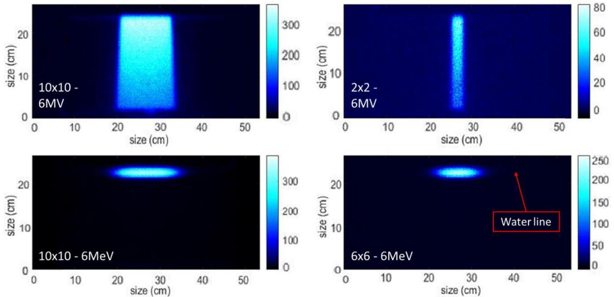
Figure 4: Water tank phantom images with different beam parameters. On top X-ray beams - a) 10x10cm b) 2x2cm, on the bottom electron beam - c) 10x10cm d) 6x6cm.
