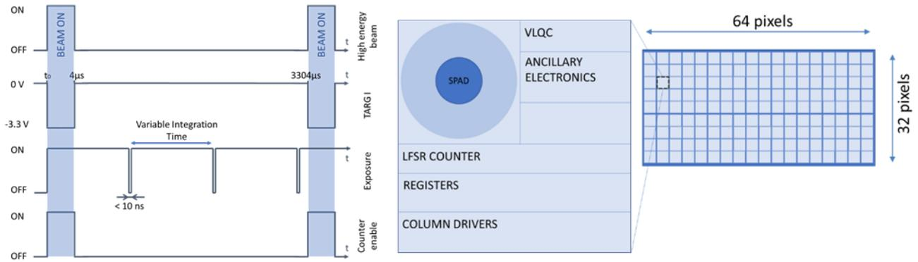
Figure 1: Left: Acquisition timing diagram of the SPC3 camera. Right: SPC3 pixel organisation schematic
