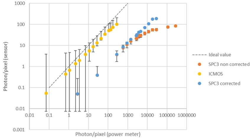
Figure 3: ICMOS and SPAD sensitivity curve with normalized scale. Blue curve corresponds to the dead time corrected signal.
